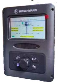
The system has pre-warning, overload alarm, and overload control output functions. Stabiliser position, Crane pressure during lifting, Auto diagnostic system and Error code information for fault directions will all be displayed by the 4.3 inch with colour TFT LCD display. Said display:
